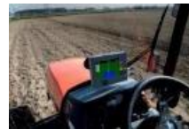
Straight-line assistance for agricultural vehicles to reduce the burden of working on the farm
