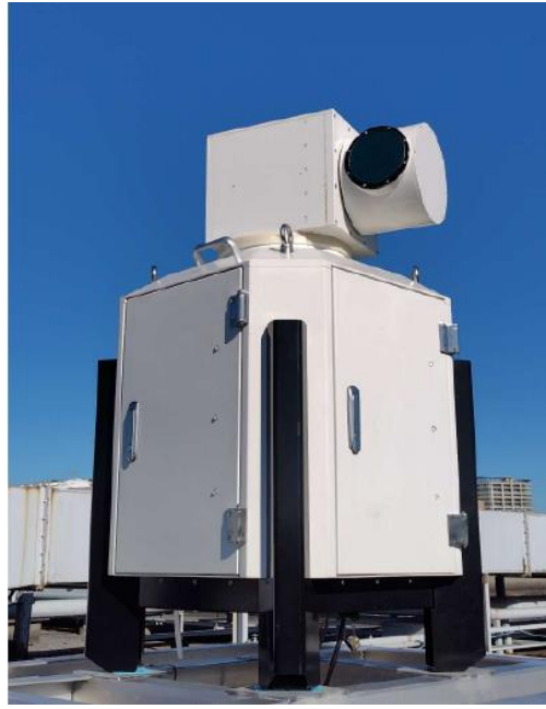
Doppler LiDAR during wind condition observation (Installed on the TOKYO KEIKI Headquarters rooftop and performed the test until the end of June 2025)
