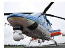
Antenna directioning systems which continuously grasp the position and attitude directions of helicopters, control relay antennas toward receiving stations, and transmit video without interruption
