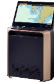
Electronic Chart Display and Information Systems (ECDIS) that display navigational charts in real time
