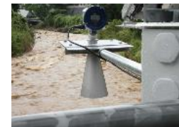
Level gauge that monitors river flooding
