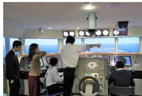
ECDIS (Electric Chart Display and Information Systems) that display navigational charts in real time
