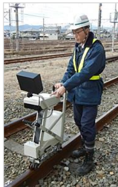
Ultrasonic rail flaw detector that pinpoints flaws more efficiently than rail inspection cars
