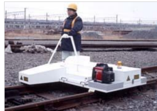
Switch profile gauge that simultaneously measures rails wear, crossing wear, and track geometry
