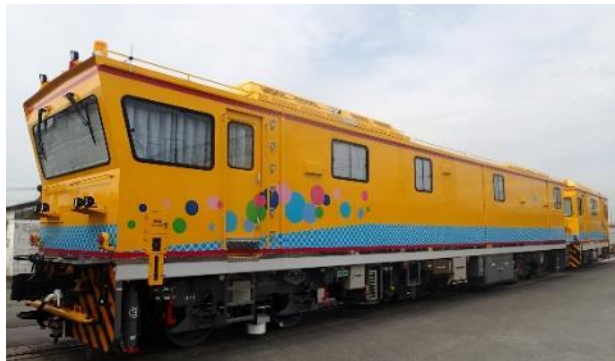
Ultrasonic rail inspection car that performs non-destructive inspections using ultrasonic wave.
