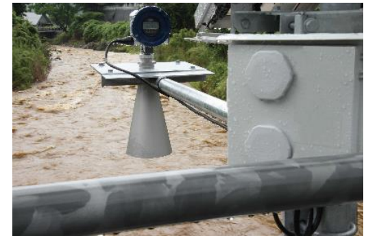
Crisis management water gauges that provide early detection of rising river levels
