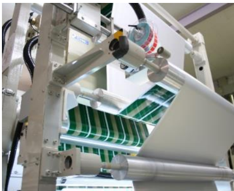
Print inspection system that ensures print quality by detecting print-defects
