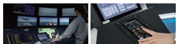
The joystick controller installed in the onshore emergency response block. The autopilot can be controlled by simply moving this small control lever.
