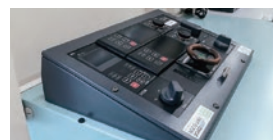
The PR-9000 autopilot installed onboard the container ship "SUZAKU"
