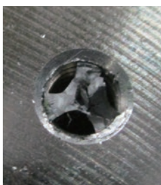
Broken tap drill bit
