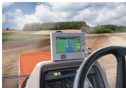
Automated straight-line assistance device for agricultural vehicles
