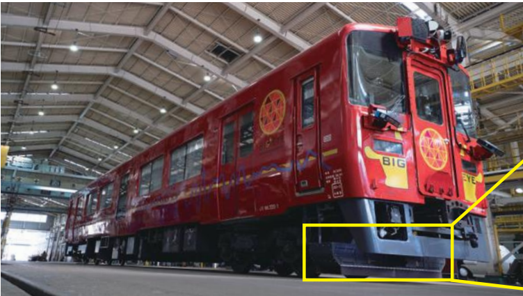
A multifunction inspection car of Kyushu Railway Company (JR Kyushu) equipped with the track diagnosis support system
