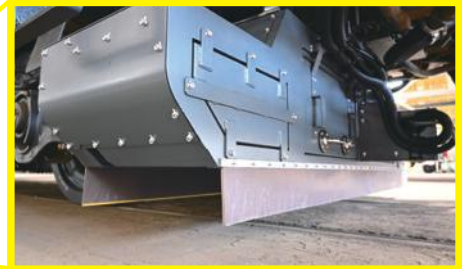
Track diagnosis support system
