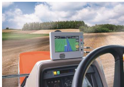
Automated straight-line assistance device for agricultural vehicles
