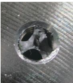
Broken tap drill bit
