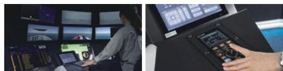
The joystick controller installed in the onshore emergency response block. The autopilot can be controlled by simply moving this small control lever.
