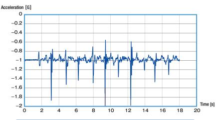
\*Lower peaks reflect the impact of the foot as it comes into contact with the floor.
