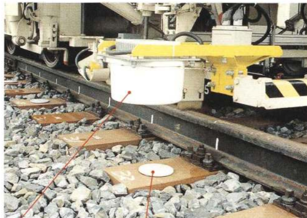
DD Reader on vehicle, DD Memory (DD-1) on sleeper Application on Multiple Tie Tamper
