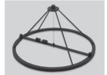
●方位鏡 Azimuth mirror
